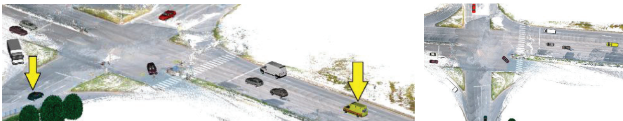
Fig. 12 3D point cloud with high density from accident scene [authors]
