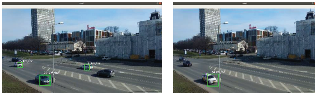
Fig. 8 Speed estimation within ROI(left), outside ROI(right)
