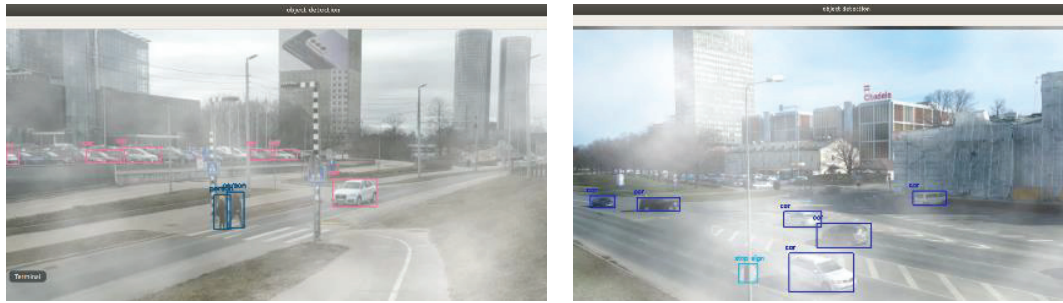
Fig. 4 Object detection with fog filter = 50%(left) and 70%(right)
