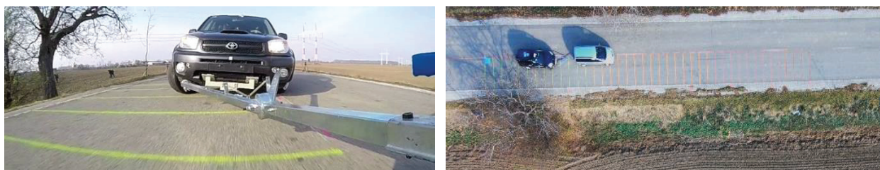
Fig. 5 Maximum steering angle of 7 meters after vehicle disconnection
