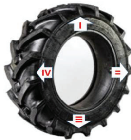
Fig. 1 Marking the index points of the mini-tractor's wheel
