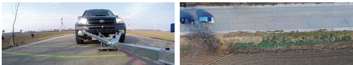
Fig. 4 Moment of disconnection of the synchroniser on the disconnection plate
