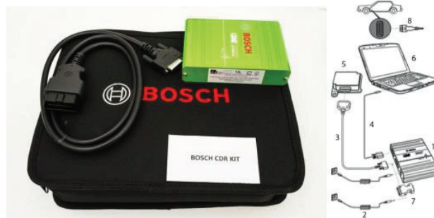
Fig. 1 Bosch CDR Kit (left) and its wiring diagram (right, [1])
