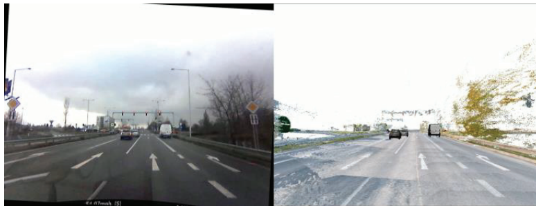
Fig. 14 Record from dash board video device and from simulation 32 seconds before collision [authors]
