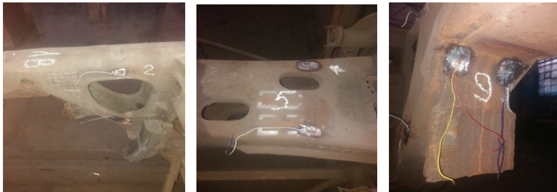
Fig. 3 Installation of strain gauges on experimental cars
